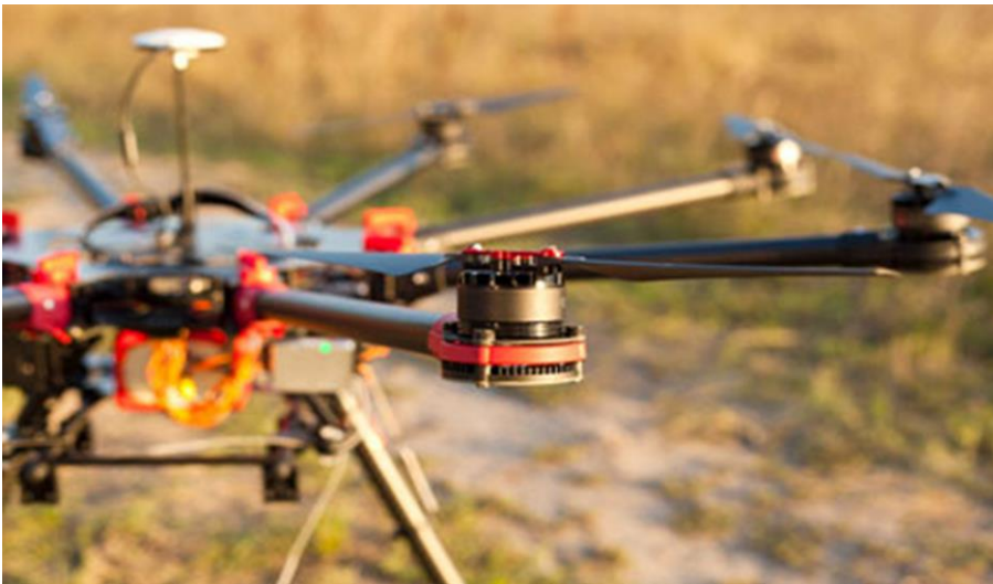
Workswell WIRIS thermal imaging system located on the drone. The system combines a thermal imaging camera and a camera in a visible spectrum.
