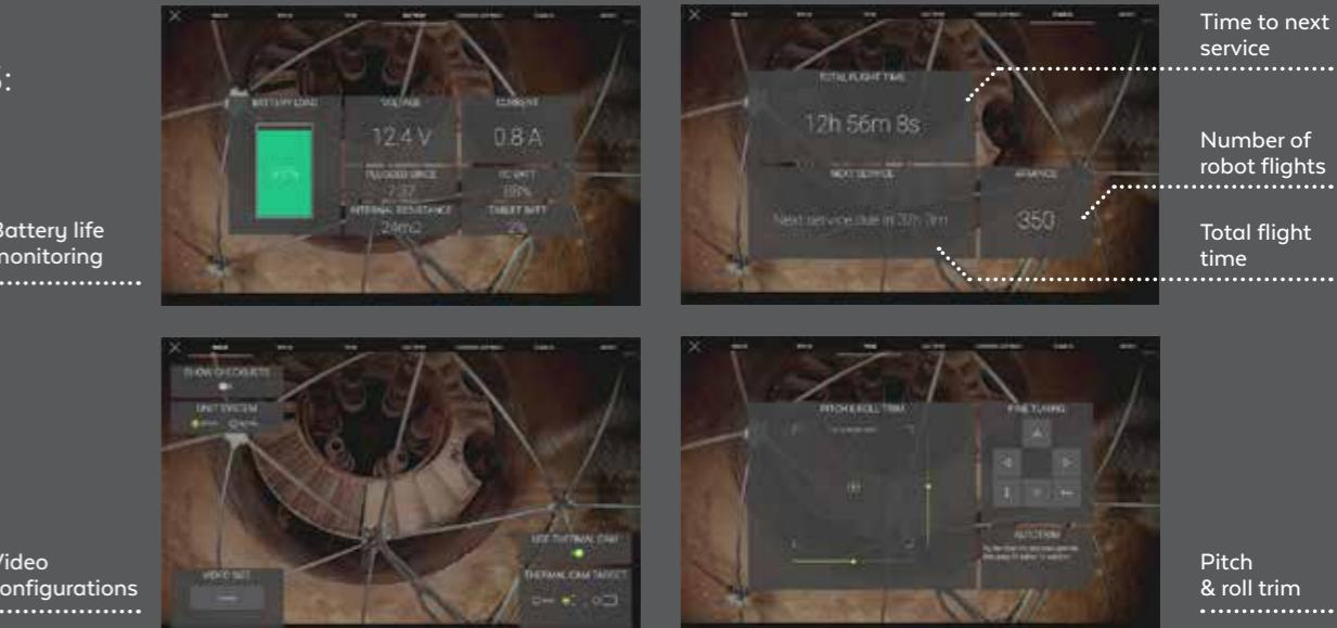
In addition to displaying the live SD stream received from the drone, Elios Cockpit displays live telemetry data, gives you access to a detailed status of your drone and let you adjust settings right from the application.
