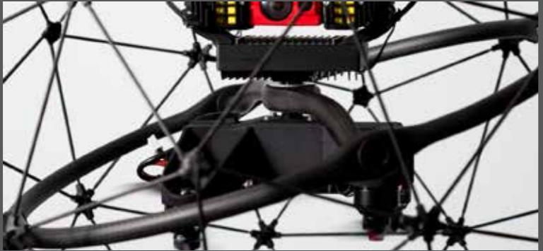
The protective frame of Elios is no ordinary one. It is decoupled on three axes from the inner frame - the drone - using a gimbal mechanism. This ingenious decoupling mechanism is what allows Elios to remain stable in the event of a collision.
