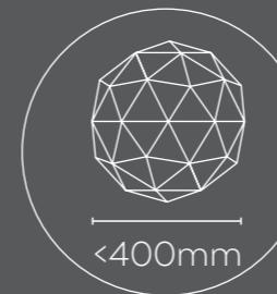
Spherical, the protective frame comes in one size only. With a diameter just below 400 mm, it is slightly smaller than the smallest standard manhole.
