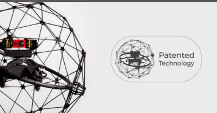
Patented by Flyability, the protective frame is a unique and pragmatic approach to flying indoors, in complex and confined spaces and in contact with people. Discarding the need to sense and avoid obstacles, you can start inspecting and exploring - without waiting - the hardest places to reach.
