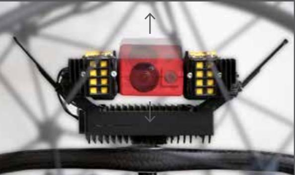
Mounted on a rotatable head the cameras can capture images looking above and below the drone. The full HD camera offers a total field of view of 215° and a horizontal field of view of 130° while the thermal camera offers a total vertical field of view of 182° and a horizontal field of view of 56°.
