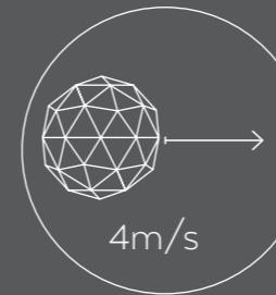
Elios' protective frame is made up of carbon fiber covered with a soft coating. It can sustain collisions, evenly, all around the drone at a speed reaching up to 4 m/s.
